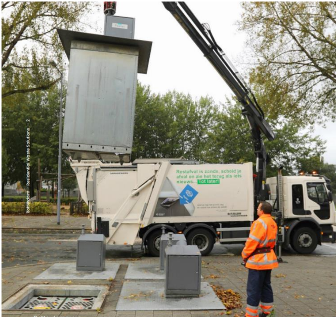
Figure 3. Underground container system
